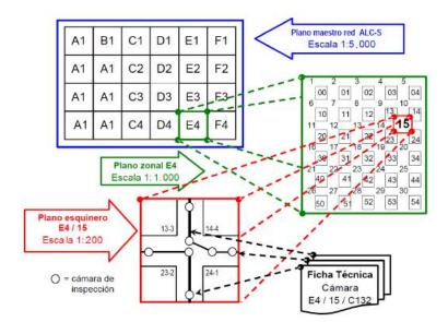
For further guidance, the following figure presents the set of plans and datasheets that form the register of ALC networks.
