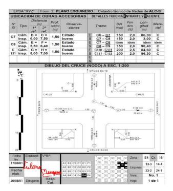
As seen in the "details" part of the above figure, a section of pipe that enters and leaves a support work (structure), is identified by indicating the two structures which that section connects. It is a convention that the order of the two N  $^{\circ}$  ID goes from left to right according to the flow rate direction.
