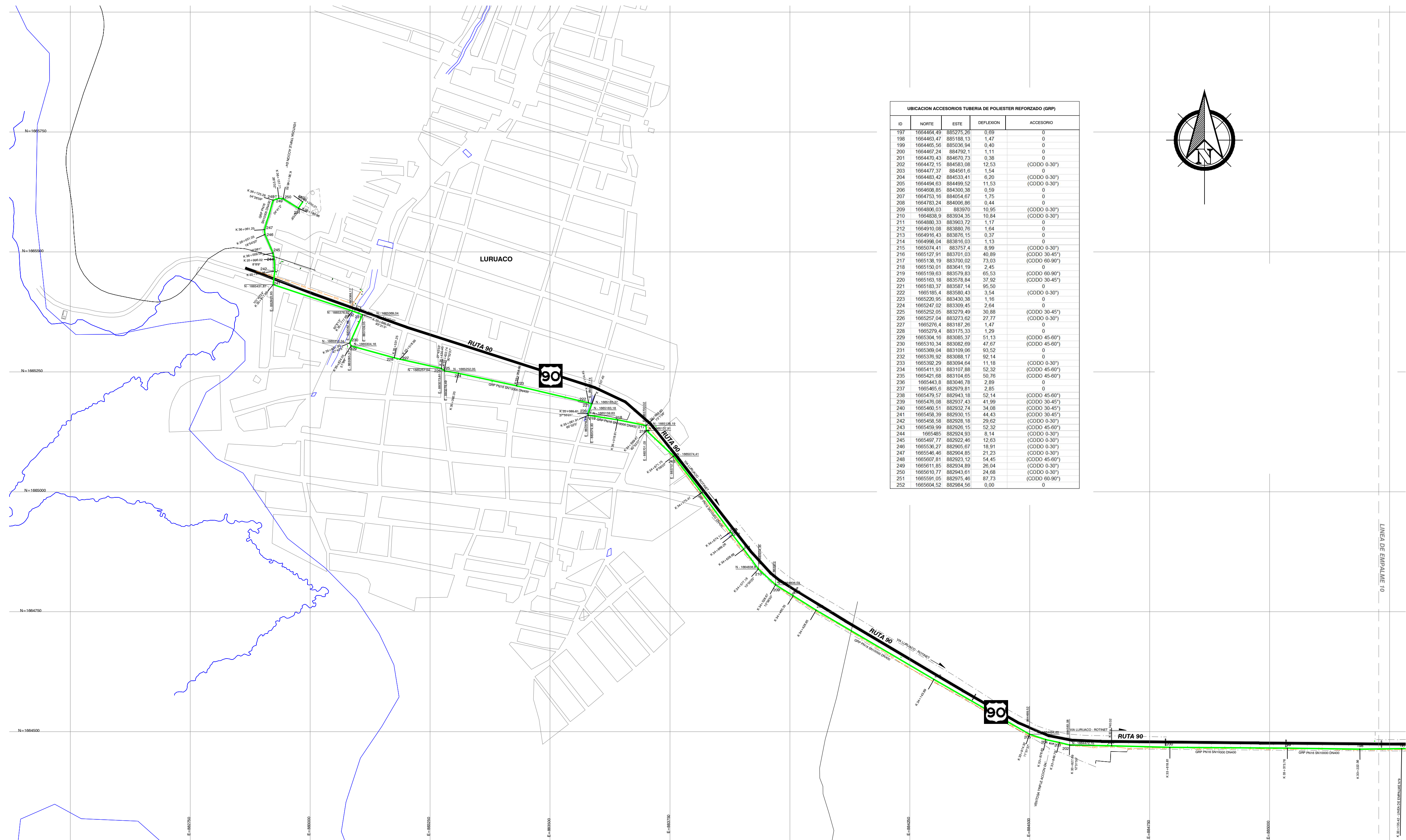
PLANTA TRAMO - SECTOR IO K33+135.42 a K36+220.00 TUBERIA GRP PN16 SNI0000 DN 400 ESC. 1:5000
