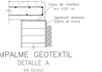
EMPALME GEOTEXTIL DETALLE A SIN ESCALA
